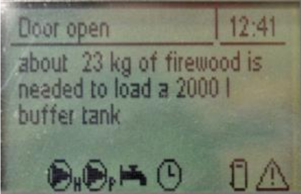
Fill assistance based on thermal storage volume and temperature
