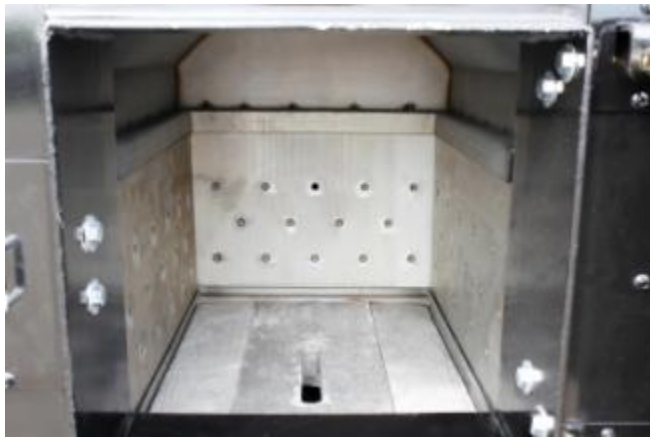
Firebox cladding and distributed primary air.
